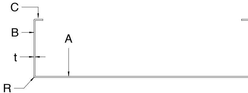
② LIPPED C PROFILE SECTION DETAIL 1 : 1
